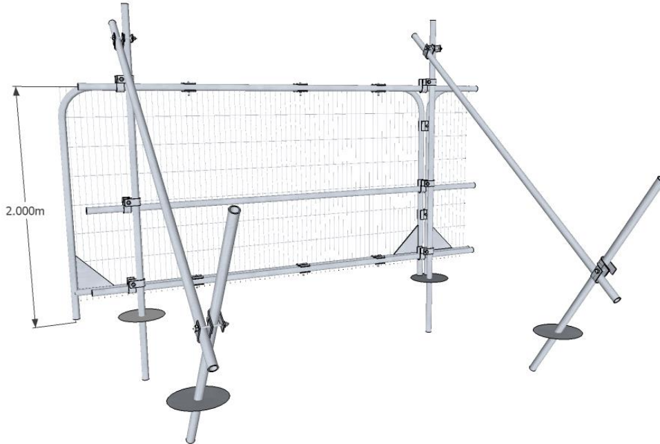
Figure 1. Protective fence specification
